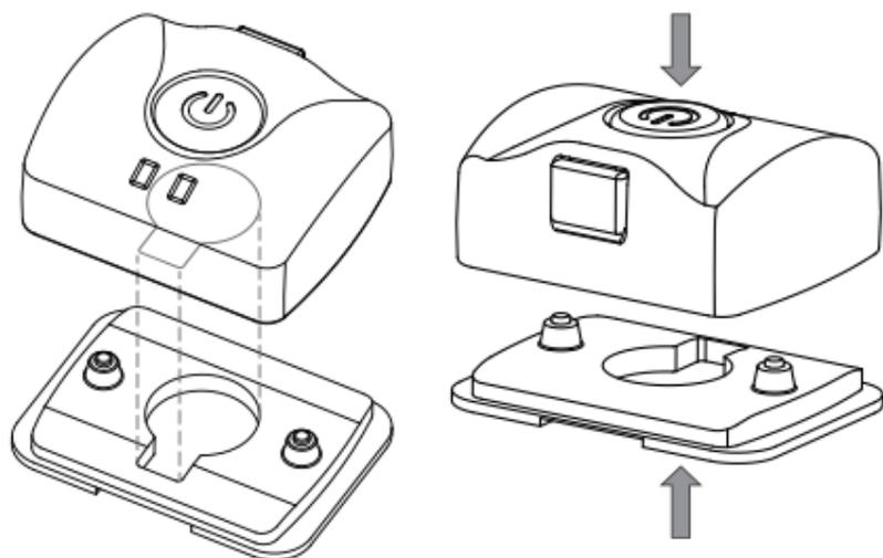
**Figure 12. Connecting the stimulator to the electrode pad**
