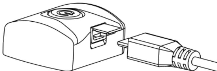
Figure 9. Connect the USB cable to the stimulator.
